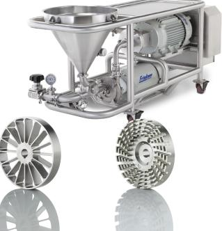
The Fristam Powder Mixer provides quick, highperformance blending of wet and dry ingredients into a fluid stream. It incorporates the uniform powder induction of the FZX liquid ring pump and thorough blending of the FS Shear Blender into a single, compact system. Powders can be wetted and dispersed on the first pass, dramatically reducing process times.
